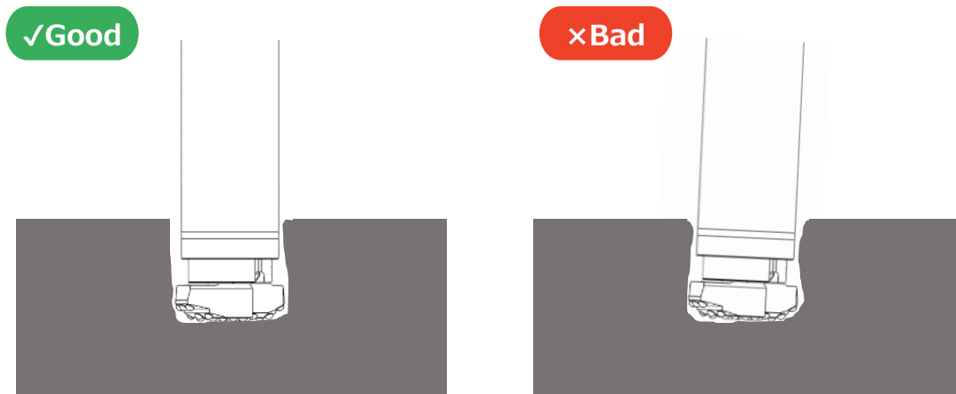
Figure7: Checking the casing pipe alignment
